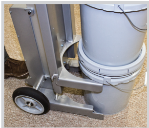
Lifting yoke holds pails in place.
