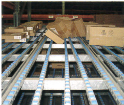
Individual tracks can cause carton hang-ups.
